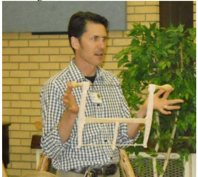
Eric Lamp: Traditional Bow Saw he made. Some of the parts he got from Gramercy tools. He explained how the curved bows help with the tensioning of the sawblade.
