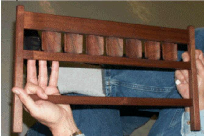
The panels in the field of the headboard are trapezoidal, fully coved and mortised into the horizontal rails. His technique for cutting the cove was using a series of progressively stepped dado passes, as tablesaw coving would not create a large radius. Les Hastings suggested using a router jig to shape the cove.
