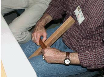
He then showed us how to tune and use a hand scraper to tame the wild grain that a hand plane wills tearout. A scraper should be cutting curl shavings; not dust if it is has the correct burr turned. The steeper you are presenting the scraper to the workpiece, the duller the tool and it is time to tune it up. He suggested that you use thumb gloves to keep your fingers from being burned as scraping creates lots of heat!
