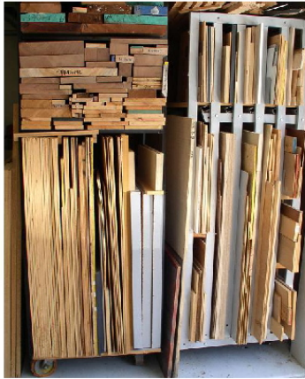
Sheet good / small cutoffs storage racks on wheels
