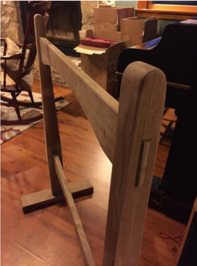
Ron Jackson showed his twin screw vise (sometime called a Moxon vise). This was a project that the “Hand tool Special Interest Group” worked on last month. The screws were made with 1 inch ACME thread stock. The adjustment knobs were fabricated from plumbing end caps epoxied onto the ACME thread nuts. The ACME threads allow the nuts to tighten and loosen more rapidly.
