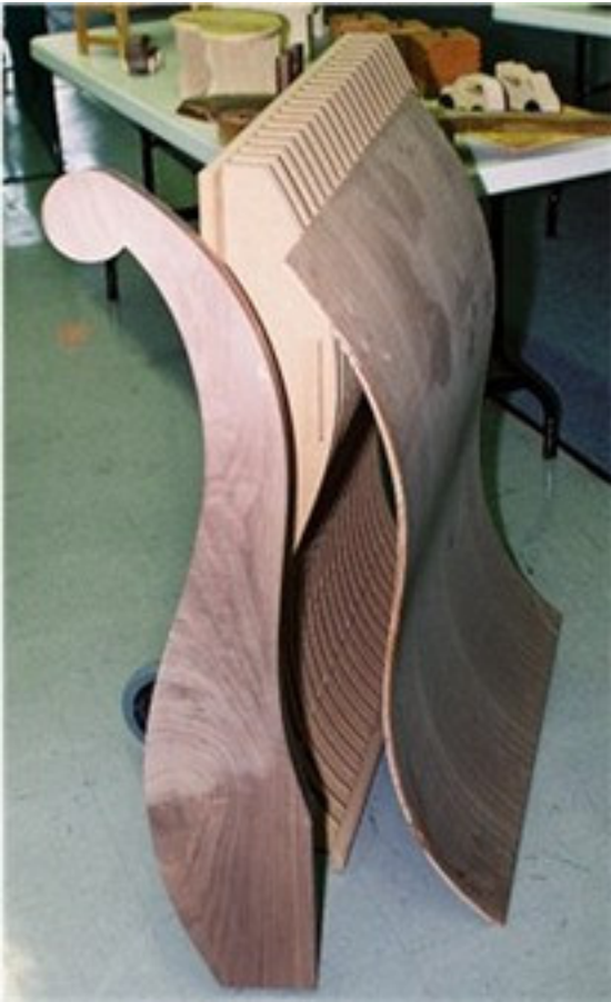
Bending form and ends for baby bed by Less Hastings
