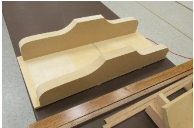
In Process cutoff sled
