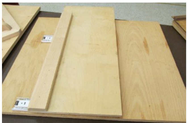
Crosscut sled utilizing drawer slides
