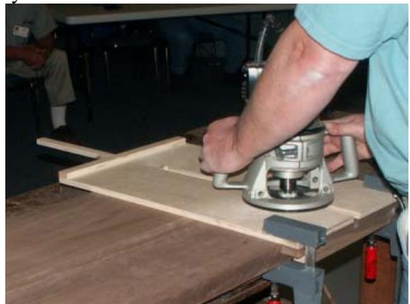
The female slot is first cut with two router passes using a template guide collar, the first hogs out most of the material, the second cleans up the cut. Les uses a parallel slot without tapers, he only glues the end of the slot away from where he starts the panel slide in i.e. the rest of the panel is held in place with the dovetail and floats.
