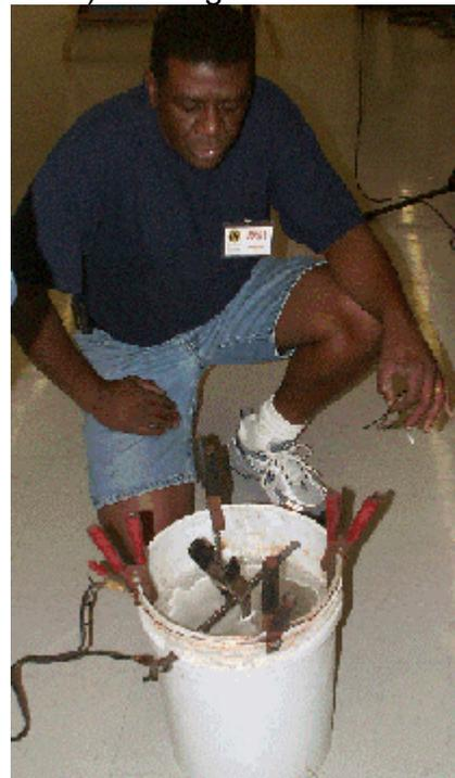
Added sacrificial electrodes and showed how to hook up the electrical connections to a battery charger so that nobody gets hurt. And then he plunked in a rusty hedge clipper half. In less than 3 hours, it was amazing how much rust was removed from the clipper and
