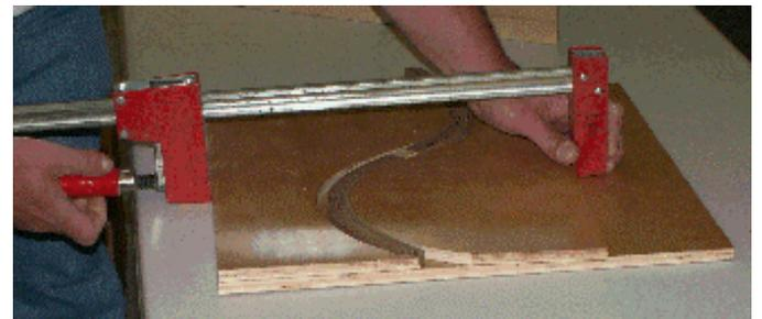
The number of plies that he will use in a shape is determined by the severity of the radius or arc. He recommended using more plies that are thin rather than trying to force heavier pieces into the shape. This, he said, will also minimize the tendency for spring back.
