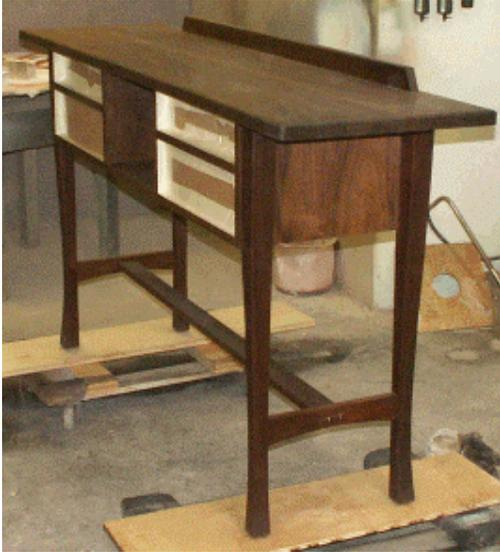
After a tack cloth wipe down, he sprayed the piece with a light coat of lacquer sanding sealer.
