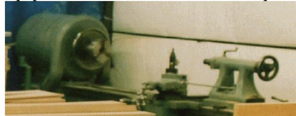
including this lathe designed to hold 9 ft long logs up to 30 inches in diameter. His other equipment is comparable.
