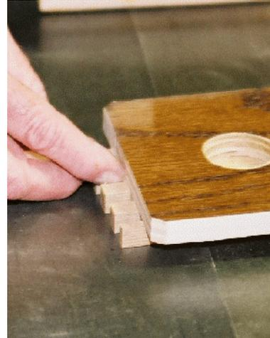
Note the clipped corners on the caul that were used to avoid gluing the caul to the workpieces.
