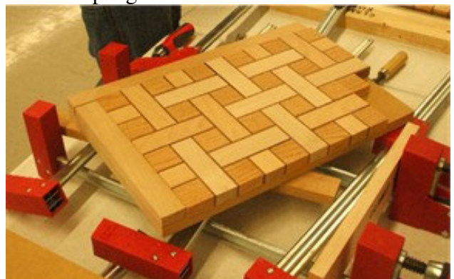
Kevin Huber's sample layup of woven breadboard ready for glue-up
