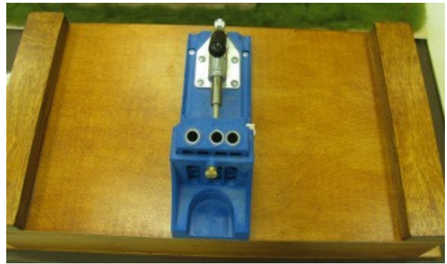
Bob Ziegfeld Krieg jig mounting jig/storage box
