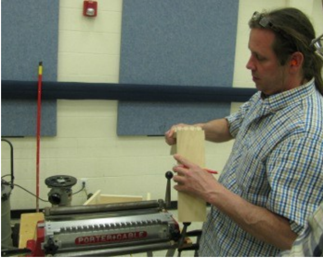
Randy Crowley with dovetail jointing jig
